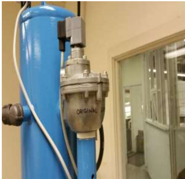
NEW 1 1/2" GOYEN PULSE VALVE UNALTERED
