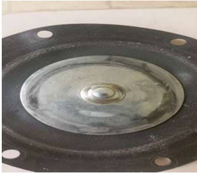
APPEARANCE OF PRIMARY TURBO DIAPHRAGM AFTER TESTING
