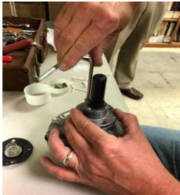
REASSEMBLY OF GOYEN VALVE WITH TURBO DIAPHRAGM REPLACEMENT KIT
