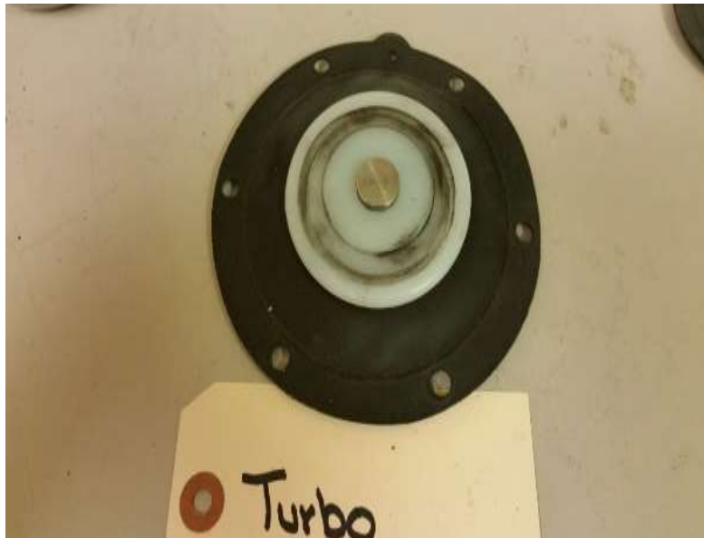
APPEARANCE OF SEAT SIDE OF TURBO PRIMARY DIAPHRAGM
