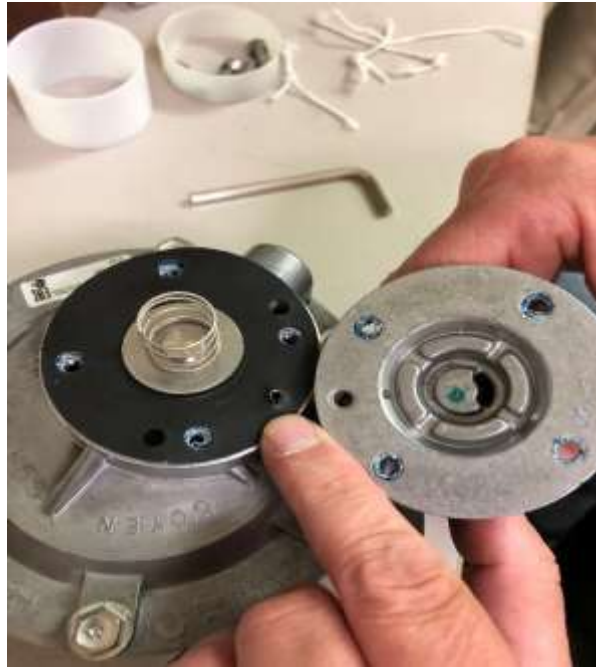
TURBO SECONDARY DIAPHRAGM REPLACEMENT
