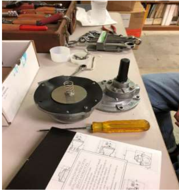
APPEARANCE OF TURBO PRIMARY DIAPHRAGM PRIOR TO TESTING
