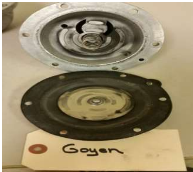
APPEARANCE OF PRIMARY GOYEN DIAPHRAGM AFTER TESTING
