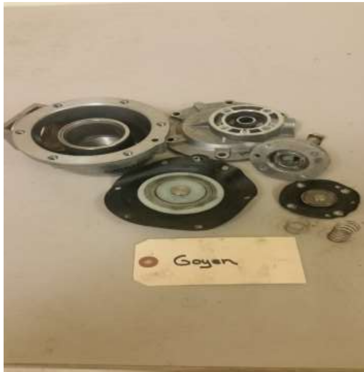
GOYEN VALVE DISASSEMBLED AFTER TESTING
