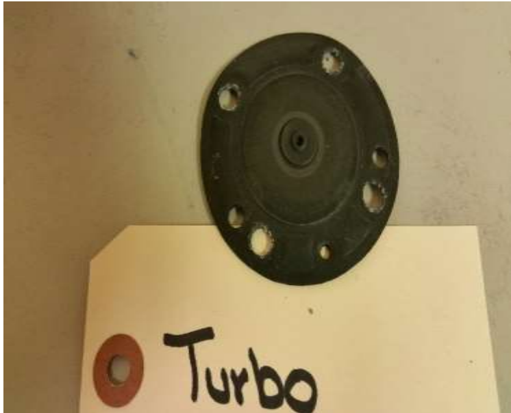
APPEARANCE OF SECONDARY TURBO DIAPHRAGM AFTER TESTING
