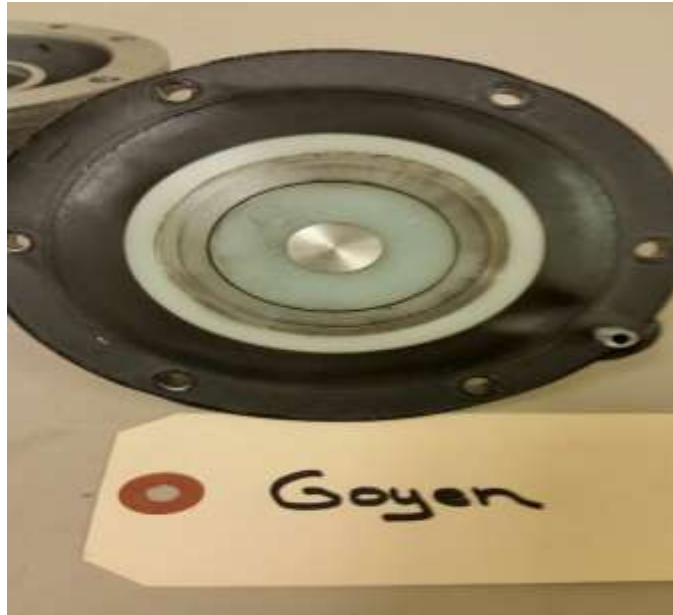
APPEARANCE OF SEAT SIDE OF GOYEN PRIMARY DIAPHRAGM
