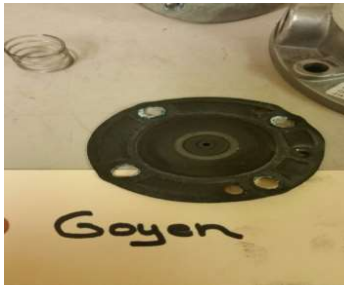
APPEARANCE OF SECONDARY GOYEN DIAPHRAGM AFTER TESTING
