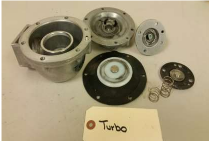
GOYEN VALVE WITH TURBO DIAPHRAGM REPLACEMENT KIT DISASSEMBLED AFTER TESTING
